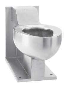
These Toilet Fixtures are designed for high security areas with an accessible pipe chase. The fixtures are fabricated using 14-gauge type 304 stainless steel, seamlessly welded to form a one piece, vandal resistant unit. Internal piping is stainless steel. Exposed surfaces are polished to a satin finish, except for the integral seat which is polished to a bright mirror finish.
