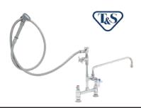
adjustable from 7-3/4" to 8-1/4" centers. Built-in check valves prevent cross flow of water. Hanger hook holds hose when not in use. Hose and spray is 78" overall. Any length hose and other length nozzles furnished on request.
