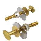
Specially designed solid brass closet bolt. 1/4" and 5/16" diameters with easy break off indent and no spin tab which sets bolt firmly in place when assembling closet bowl to flange.
