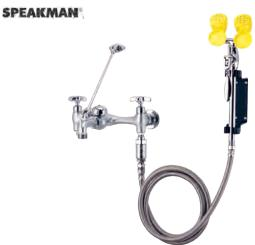
Combination eyewash/drench hose and back mounted service sink faucet. The eyewash is attached directly to the faucet's cold water integral stop cavity allowing independent operation. No risk of scalding. 6-foot stainless steel hose.
