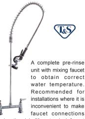
below the sink. 8" center deck faucet with union coupling connections allows faucet to be installed to the piping at sink top level. Faucet has 1/2" IPS female eccentric flanged inlets. Spring action type gooseneck gives the user a wider range of coverage. Unit is 40" high with 15" overhang and 9" clearance. Longer length hoses furnished on request.
