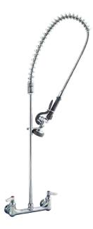
A complete pre-rinse unit. Assembly is used where a wall or splash back connection is desired. Faucet has 8" centers with 1/2" IPS female eccentric flanged union inlets. The spring action type gooseneck gives the user a wider range of coverage. Unit is 34" high with 15" overhang and measures 5" from bottom of spray valve to C/L of faucet. Longer length hoses furnished on request.
